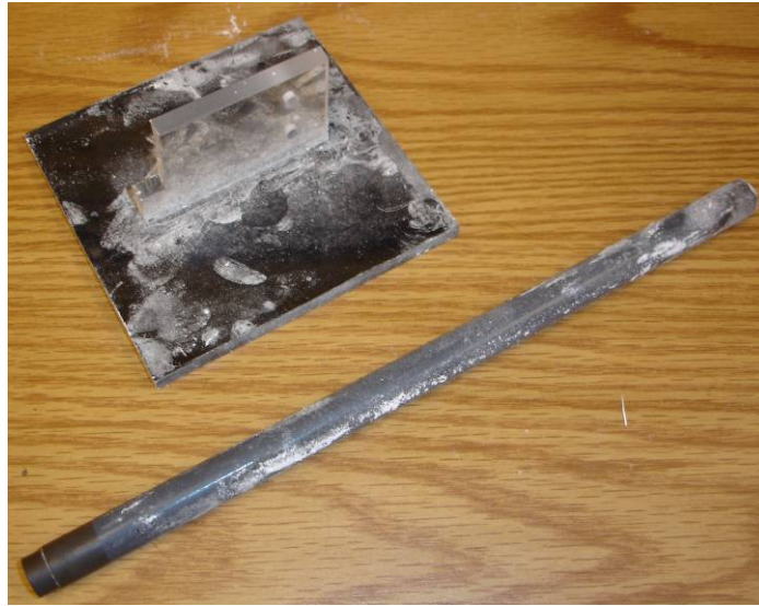
Figure B 37 Powder Spreader and Compactor
